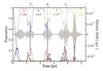
FIG. 6. (Color online) Time-dependent target: time evolution of the level populations with an optimal field (shown in gray).
