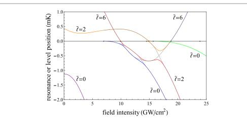
**Figure 5.** Positions of bound levels and shape resonances as a function of non-resonant field intensity for <sup>86</sup>Sr. salculated with 'universal' intensity-independent nodal lines. Avoided crossings are here clearly visible, making it impossible to match colors and labels. Diabatized curves, to which the labeling corresponds, are drawn in black dashed lines.
