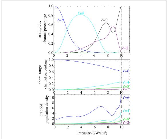
Figure 6. Hybridization of the  $\tilde{\ell}=6$  shape resonance of  $^{86}\text{Sr}^{88}\text{Sr}$  as a function of non-resonant field intensity, analogously to figure 3. The dotted—dashed line indicates the crossing with threshold.
