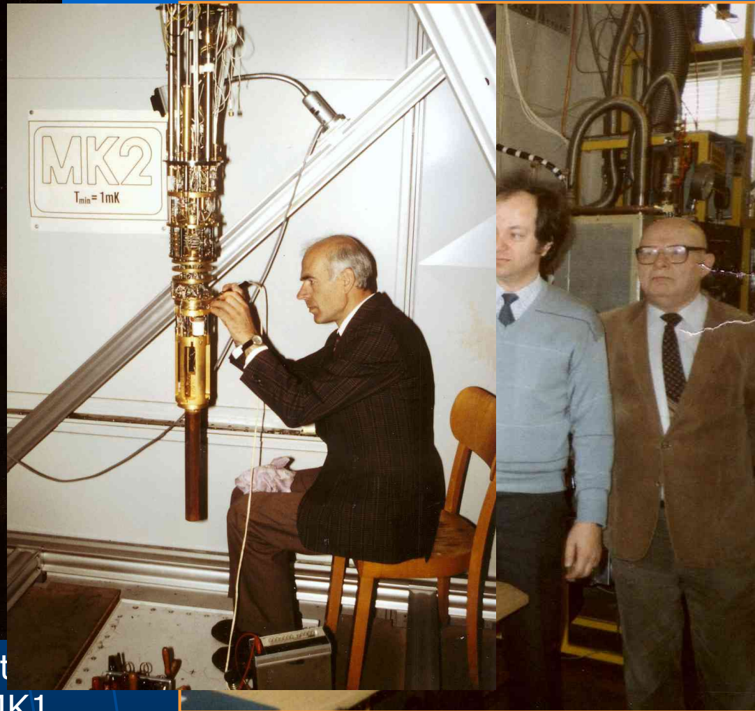
Nuclear demag stage being mounted for first test, 1987
